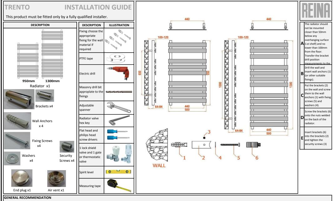
Before fitting the radiator it is necessary to wash out the heating system to remove any existing mud, scale, work residues, traces of flux, oil, etc.
